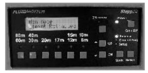
**Note:** Some buttons do double duty. These buttons step through both of the indicated bands. Each press of the button moves you sequentially through all of the pre-set frequencies for both bands in a continuous loop.
