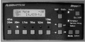
80m - 6M Controller - This is the controller used on the BigIR vertical with the 80m coil option installed.
