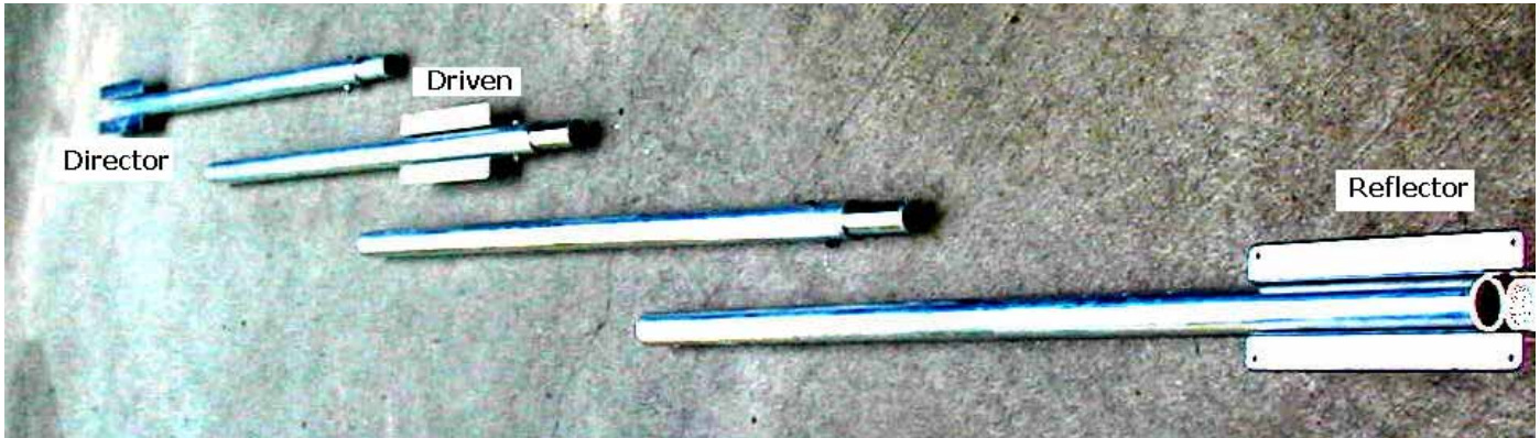
Figure 5: The four sections of a 3 element yagi shown in the staggered order of installation
