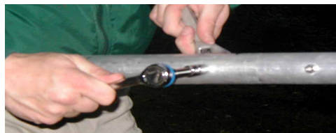
Figure 4: Securing the boom sections
